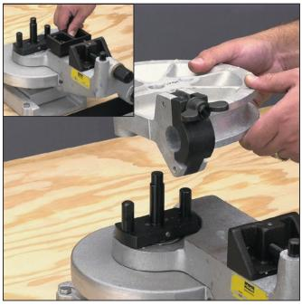
**Three Hole Blocks** — To use the larger three hole radius blocks, just install a third pin in the drive plate, if necessary, then remove the slide block vise adapter by removing the two Allen-headed screws in back of plate to provide space for the larger radius blocks.
