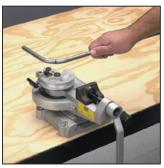
**Bends from 90° to 180°** — The 400 Series Tube Benders bend tubing up to 180° with ease. The procedure for bends over 90° is the same as for bends to 90°. See Step 4.
