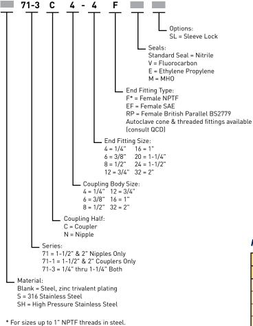
For sizes up to 1 NPFF threads in steel. For sizes up to 1" NPSF threads in stainless steel. For sizes over 1" NPT threads.
