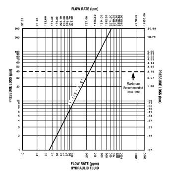
Gallons per minute (gpm) in US gallons Test Media MIL-H-6083 Hydraulic Fluid at 90°F ± 5°F (+32°C ± 1.5°C) sg .83
