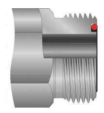
Standard O-ring in half-dovetail groove
