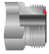
Trap-Seal in half-dovetail groove
