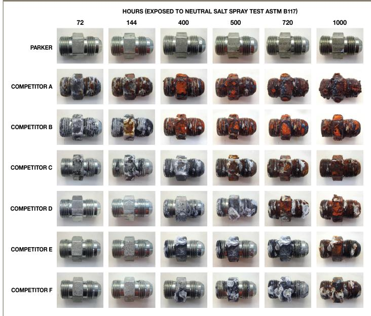
Pictures and testing were completed by Miami Valley Materials Testing Center – an accredited independent test center.
