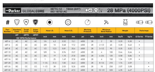
Reinforcement: One- or two-braid steel wire for sizes -4 to -12 | Four-spiral wires for sizes -16 to -24 | Six-spiral wires for size -32
