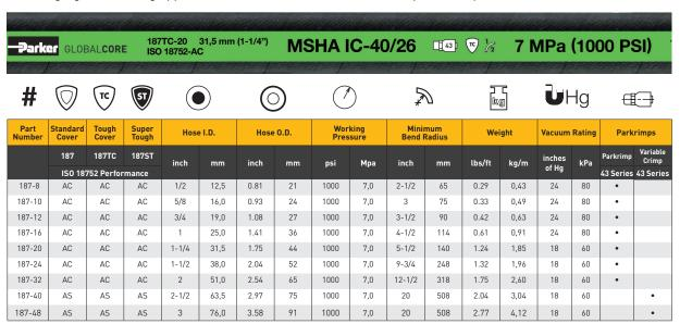
Inner Tube: Synthetic Rubber | Reinforcement: One- or two-braid steel wire
