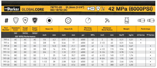
Reinforcement: Two-braid steel wire for size -4 | Four- or six-compact spiral steel wires for sizes -6 to -32
